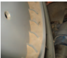
Sand build up in Oil Cooler
